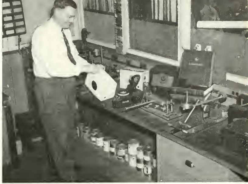
A STANDARDIZING SPECIALIST SCRATCHES A CABINET TO DETERMINE ITS WEARING QUALITY UNDER ALL CONDITIONS OF USAGE.
